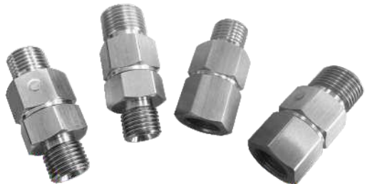
Sc01 Swivel Connector Full stainless steel, Ball bearing structure, rotate flexibly. Size: 1/4"*1/4", 3/8"*3/8", 1/4"*3/8 NPSM All available in female or male end.
