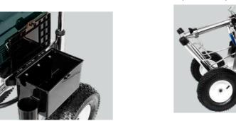
The Hanger For Side Lay The hanger is able to support the machine during reloading the material, and can also be used for hose reel during storage.
