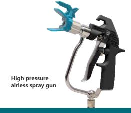
Designed for pneumatic airless paintsprayer (without filter inside.)Max.pressure: 500bar 1 7250psilnlet connector: 1/4"NPSM, 1/4"PT,M16\*1.5 Outlet thread: 7/8", 11/16", M16\*1.5
