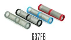
DP-637FB Airless manifold filter for Graco pumps Size: 20.6mm diameter, 91mm height DP-637FB60 black (60 mesh) DP-637FB100 blue (100 mesh)
